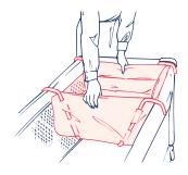
6 Pull Pocket down over floorboard to hold floorboard in place.
